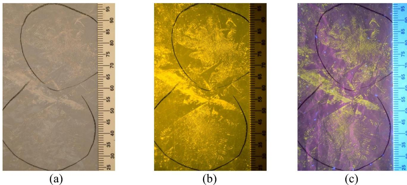
**Figure 1 - Fingermarks on a plastic bag after development with 4% Lumicyano and observed under (a) white light; (b) blue-green light (orange filter); (c) UV light (clear UV filter).**
